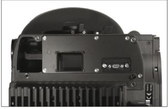
If the camera shall be used without viewfinder system, the viewfinder interface has to be protected using the viewfinder cover plate **⇔image** from the D-21 low mode support K2.70004.0 or low mode short set K2.70010.0:
