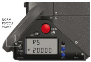
Use SEL and SET to adjust each digit. A final confirmation of the set frame rate is not necessary.
