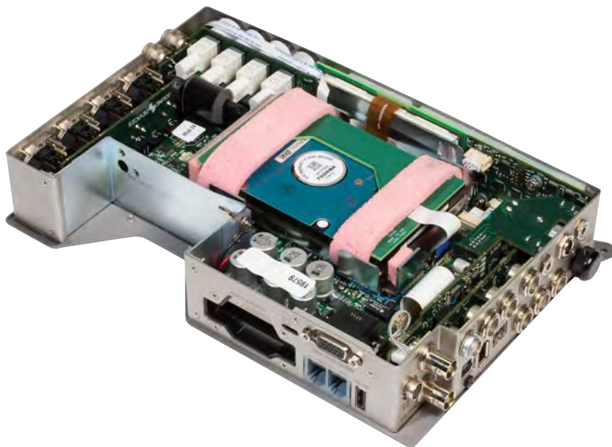
788T with bottom panel removed showing drive mounting location
